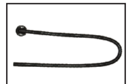
Cable loop - to protect exposed cables
